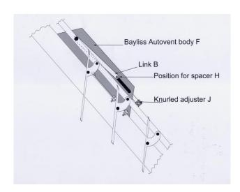
At this stage carefully insert the glass louvre blades into the sockets at each end
